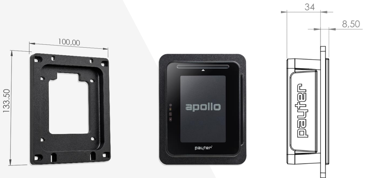
Figure 14: Dimensions ApolloMax terminal with frame
