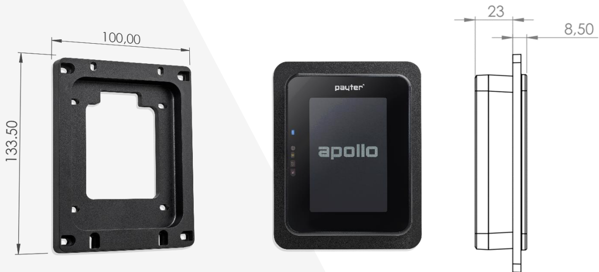
Figure 11: Dimension Apollo terminal without frame
